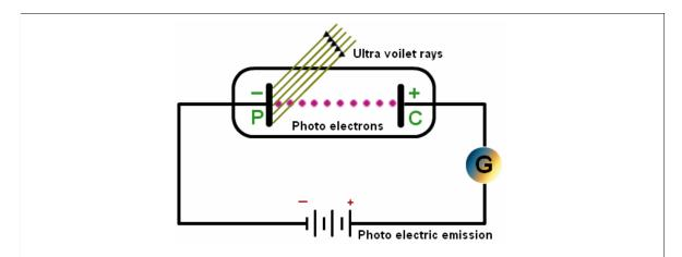
Figure 20: The experimental setup for the photoelectric effect. A voltage is applied so that the emitted electrons are accelerated towards the collecting **anode**, C. The photoelectric current is measured by the galvanometer, G. The stopping potential is determined by reversing the potential so that it retards the (negatively charged) electrons.
