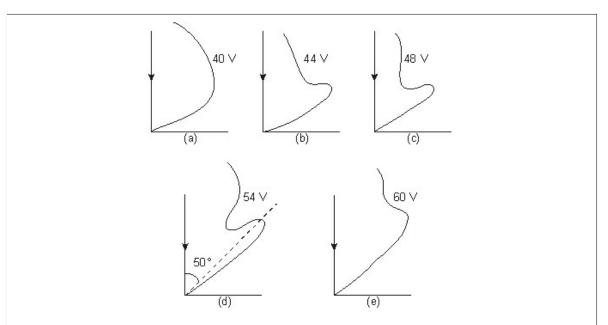
Figure 27: The results of the Davisson-Germer experiment for several different accelerating potentials. The distance of the line from the origin at some angle,  $\phi$ , to the vertical is proportional to the intensity of the scattered electrons at a scattering angle  $\phi$ . The bulges occur at angles that indicate the scattering angle corresponding to the first diffraction maximum of the matter waves of the electrons scattered off a nickel crystal target.
