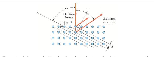
Figure 28: A diagram showing that the relation between the electron scattering angle,  $\phi$  and the angle between the incident electrons and the crystal lattice planes,  $\theta$ , is given by  $\theta = 90^{0} - \phi/2$ . Therefore the first diffraction maximum occurs at  $d \cos\left(\frac{\phi}{2}\right) \lambda$ , where  $\lambda$  is the de Broglie wavelength of the incident electrons.
