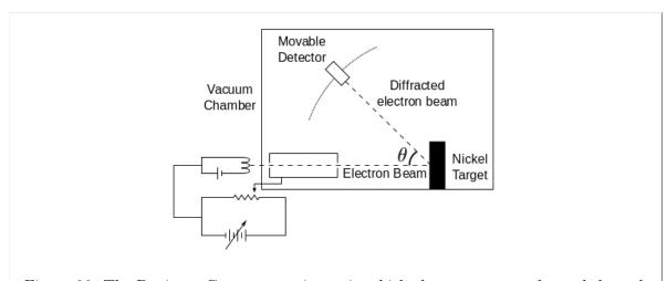
Figure 26: The Davisson-Germer experiment in which electrons are accelerated through a given voltage and then scattered from a nickel target. The intensity of the scattered electrons is measured by a detector which was moveable so that different scattering angles can be probed.
