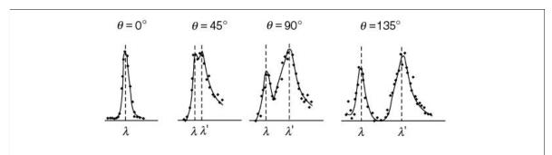
Figure 22: Incident and scattered X-ray wavelengths for various different scattering angles.
