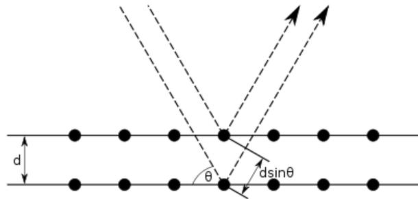
Figure 25: The path difference between waves reflected from adjacent planes of a crystal with separation,  $d$ , is (using a little trigonometry)  $2d \sin \theta$ , where  $\theta$  is the reflection (equal to the incident) angle, as shown.
