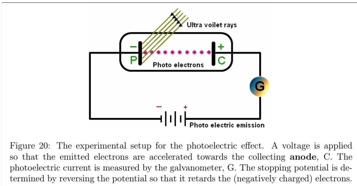
Figure 20: The experimental setup for the photoelectric effect. A voltage is applied so that the emitted electrons are accelerated towards the collecting **anode**, C. The photoelectric current is measured by the galvanometer, G. The stopping potential is determined by reversing the potential so that it retards the (negatively charged) electrons.
