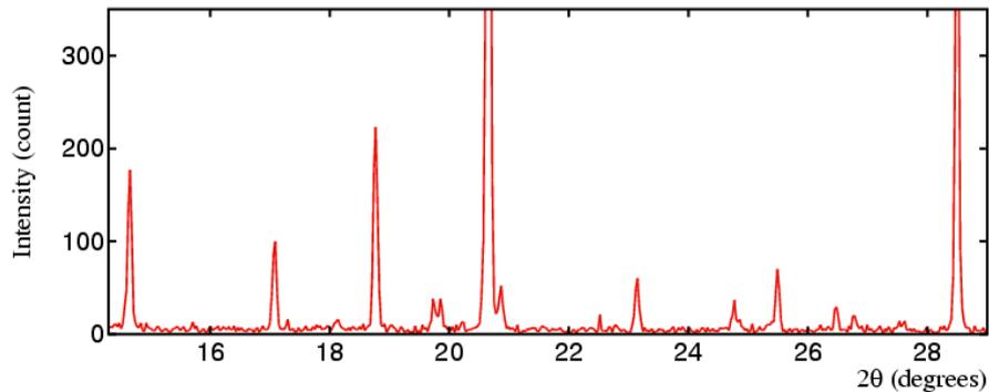
Figure 24: Diffraction maxima from X-rays diffracted from a regular crystal.
