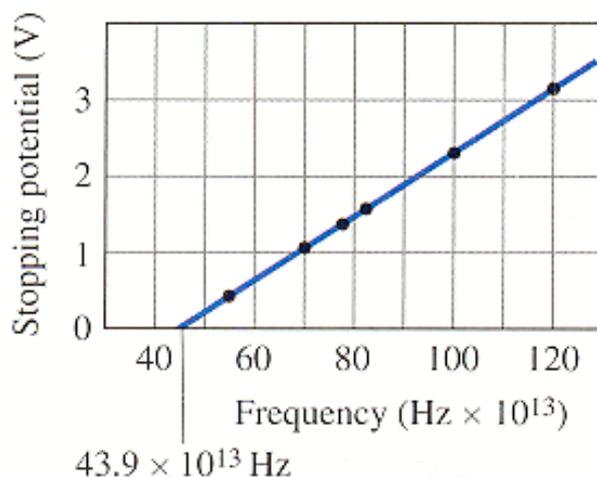
Figure 21: The result of Millikan’s experiment on the photoelectric effect showing the stopping potential against the frequency of incident radiation. The slope,  $\Delta V/\Delta f$  is Planck’s constant divided by the electric charge of the electron. The intercept is equal the work function divided by Planck’s constant.
