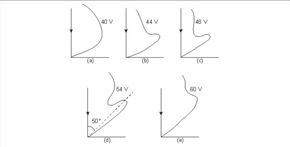
Figure 27: The results of the Davisson-Germer experiment for several different accelerating potentials. The distance of the line from the origin at some angle,  $\phi$ , to the vertical is proportional to the intensity of the scattered electrons at a scattering angle  $\phi$ . The bulges occur at angles that indicate the scattering angle corresponding to the first diffraction maximum of the matter waves of the electrons scattered off a nickel crystal target.
