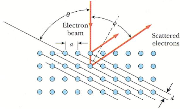
Figure 28: A diagram showing that the relation between the electron scattering angle,  $\phi$  and the angle between the incident electrons and the crystal lattice planes,  $\theta$ , is given by  $\theta = 90^\circ - \phi/2$ . Therefore the first diffraction maximum occurs at  $d \cos(\frac{\phi}{2}) = \lambda$ , where  $\lambda$  is the de Broglie wavelength of the incident electrons.
