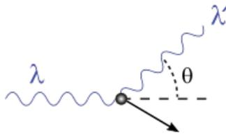
Figure 23: A photon with wavelength  $\lambda$  scatters off an electron with scattering angle  $\theta$  between the directions of the incident photon and the scattered photon. The scattered photon has a longer wavelength  $\lambda'$  since some of its momentum has been imparted to the target electron.
