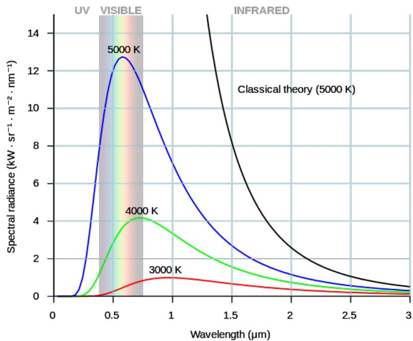
Figure 18: The intensity of radiation emitted from a blackbody in a small interval of wavelength between  $\lambda$  and  $\lambda + d\lambda$ , at temperatures of  $5000^{\circ}\text{K}$  (blue line),  $4000^{\circ}\text{K}$  (green line), and  $3000^{\circ}\text{K}$  (red line). The black line is the result at  $5000^{\circ}\text{K}$  using classical thermodynamics in which the average energy of each wave at temperature  $T$ , is  $k_B T$  for any wavelength.
