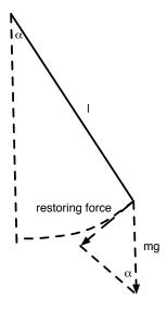
The Taylor expansion is *very* powerful! Consider the simple pendulum above. The restoring force is  $mg\sin(\alpha)$  and so the correct equation of motion for the pendulum is:
