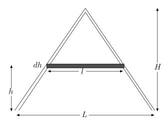
Since the length, l of the side of a slice decreases linearly with height, from l = L at height h = 0, to l = 0 at h = H, where H and L are the height and base length of the pyramid, respectively, l is given by
