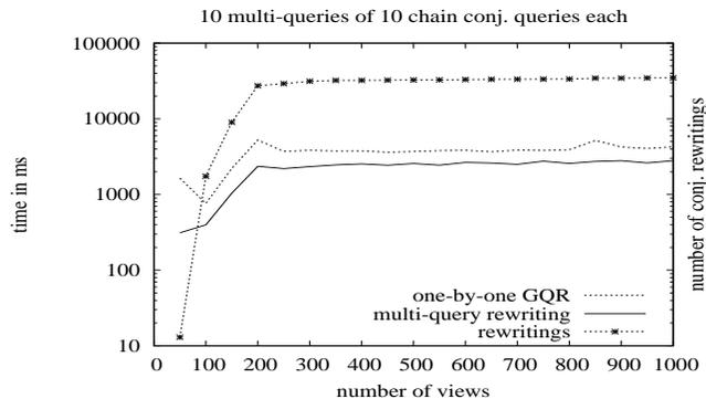
**Figure 3: Average online time and number of rewritings for 10 chain queries over up to 1000 views. The MGQR multiquery rewriting algorithm outperforms GQR rewriting queries one by one. Offline times are the same for both algorithms (not shown).**
