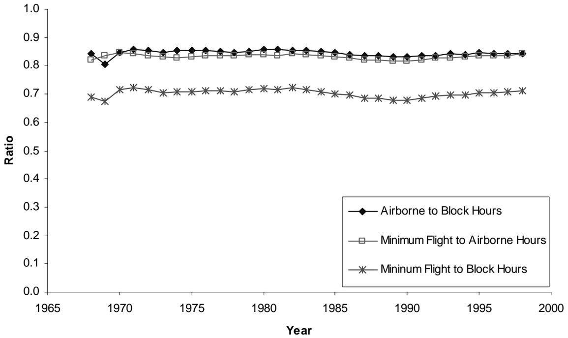
**Figure 6.2: Historical Trends in Ground, Airborne, and Total Flight Time Efficiencies**
