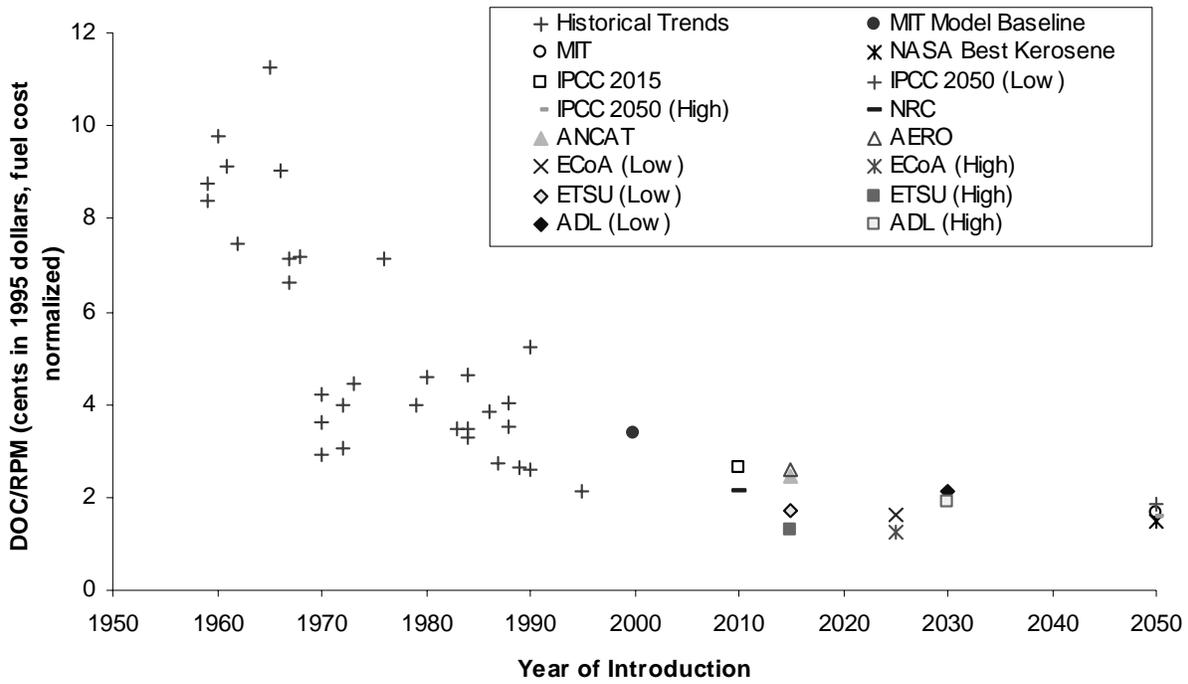
**Figure 6.6: Projected Direct Operating Costs for Future Aircraft**
