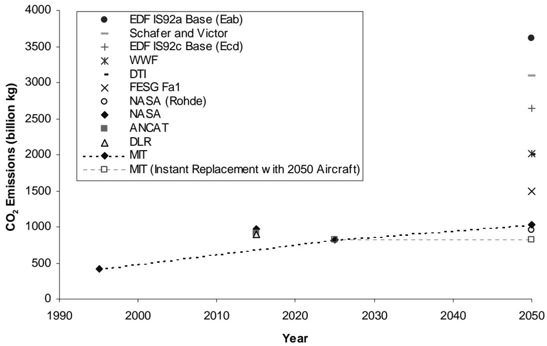
**Figure 6.9: Various CO<sub>2</sub> Emissions Growth Forecasts**
