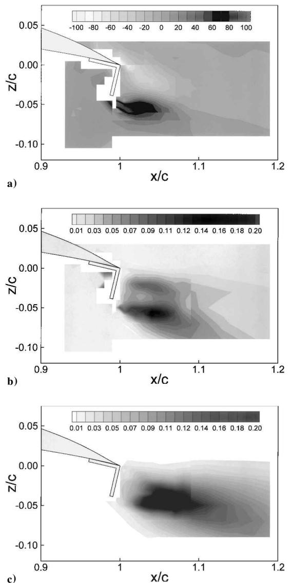
**Fig. 8** Time-averaged LDA results: a) contours of planar vorticity,  $\zeta c/U_\infty$ , b) contours of  $\overline{u'^2}/U_\infty^2$ , and c) contours of  $\overline{w'^2}/U_\infty^2$  (4% Gurney,  $\alpha = 0.0$  deg).
