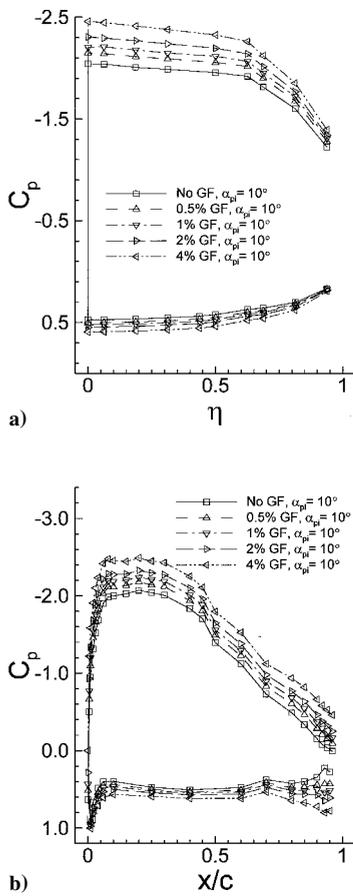
Fig. 4 Surface pressures at  $\alpha = +10.0$  deg: a) spanwise and b) chordwise.
