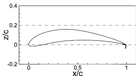
Fig. 1 Section e423 with 4% Gurney fitted,  $\alpha = 0$  deg.
