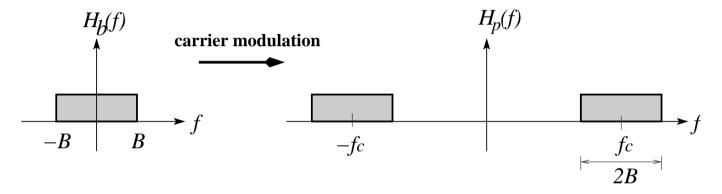
Baseband channel bandwidth  $B \leftrightarrow \text{passband}$  channel bandwidth 2B
