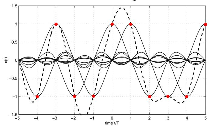
ullet At receiver, sampling at correct symbol rate enables recovery of transmitted x[k]
