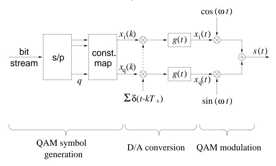
Note: e.g., odd bits go to form  $x_i(k)$  and even bits to form  $x_q(k)$ ;  $x_i(k)$  and  $x_q(k)$  are in-phase and quadrature components of the  $x_i(k) + jx_q(k)$  QAM symbol;  $x_i(k)$  and  $x_q(k)$  are M-ary symbols
