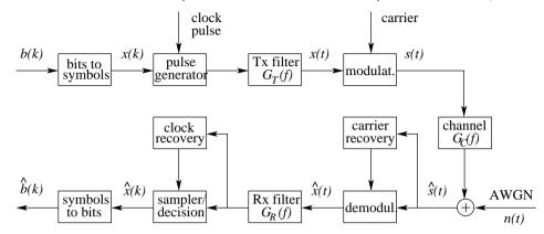
• This is for the **ideal** AWGN channel. If the channel is **dispersive**, then **equaliser** is required at receiver
