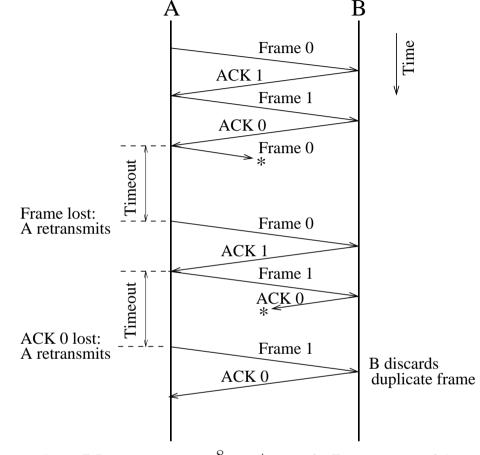
• For an LAN with R=10 Mbps and d=1 km, using  $V=2\times 10^8$  m/s and L=500 bits, a=0.1 and stop-and-wait procedure has U=0.83, which has adequate line utilisation But for a satellite link, link utilisation for stop-and-wait procedure may only be U=0.001 or lower, which is clearly wasteful
