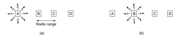
**Exposed station problem**: when B is transmitting to A, if C senses medium, it hears an ongoing transmission and falsely concludes that it may not transmit to D, but in fact it can safely do so
