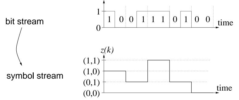
• Symbol rate is half of bit rate; symbol stream is then pulse shaped, carrier modulated, ... (what happens to required bandwidth?)
