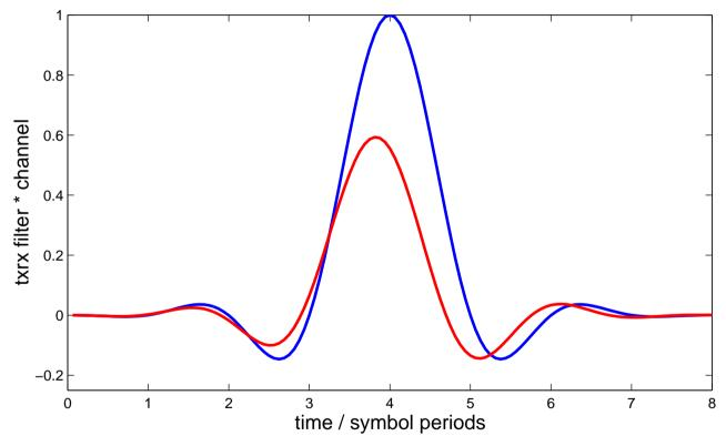
• For non-ideal channel, the combined Tx-filter – channel – Rx filter has lost the property of a Nyquist system, no longer has regular zero crossings at symbol spacing
