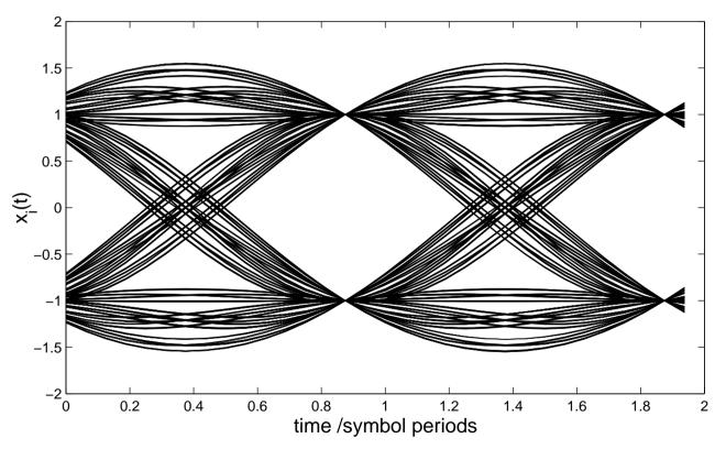
• This is called an eye diagram; ideal sampling of  $\hat{x}_i(k)$  will sample the crossing points  $\hat{x}_i(t) = \pm 1$  $\longrightarrow$  clock/timing recovery ( $\tau \approx 0.85T_s$  or  $t_k = kT_s + 0.85T_s$ )
