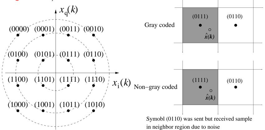
• If noise or distortions cause misclassification in the receiver, Gray coding can minimise the bit error rate
