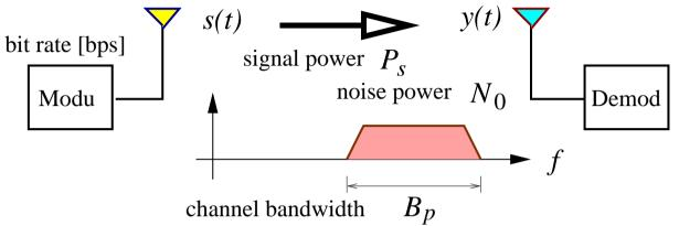
• To transmit at bit rate  $R_b$  would require baseband bandwidth  $B = \frac{R_b}{2}(1 + \gamma)$  with rolloff factor  $\gamma$ , and channel bandwidth  $B_p = 2B$
