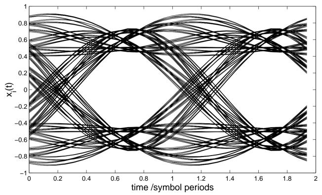
• Even with such a mild non-ideal channel, the eye diagram is distorted, this intersymbol interference together with noise effect will make the eye completely closed, leading to misclassification
