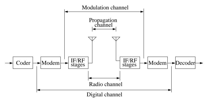
• For example, when designing decision circuit and equaliser, it is convenient to consider channel as "digital channel"
