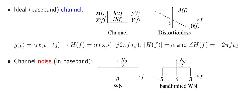
White noise has a constant PSD. Since power is area under PSD, white noise has infinitely large power. But communication system is bandlimited
