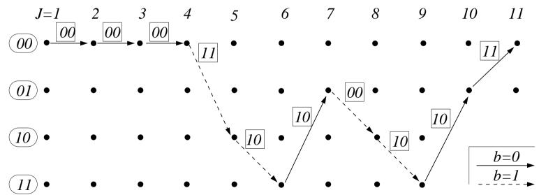
• The state is initialised at zero and as the data bit sequence enters, trellis diagram shows the history of state transitions with output bits on it
