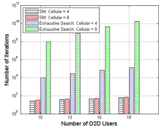
Fig. 7. Comparison of the convergence rates, in terms of the average number of iterations, required by our SM algorithm and the exhaustive search.
