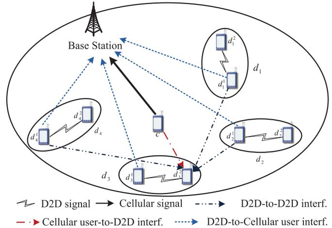
Fig. 2. Illustration of interference relationship for D2D communication underlying cellular network in single cell.
