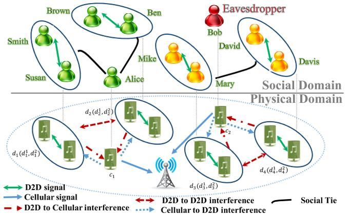
Fig. 1. A social trust aided D2D communication underlying cellular network, with 2 cellular users,  $c_1$  and  $c_2$ , and 4 D2D user pairs,  $d_1$  to  $d_4$ . In the physical domain, wireless links are subject to physical interference constraints, while in the social domain, social trusts among mobile users are indicated.
