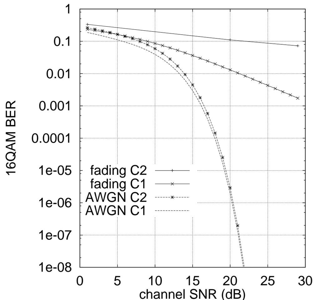
Alternatively, Monte Carlo simulation is often used to evaluate fading BER
