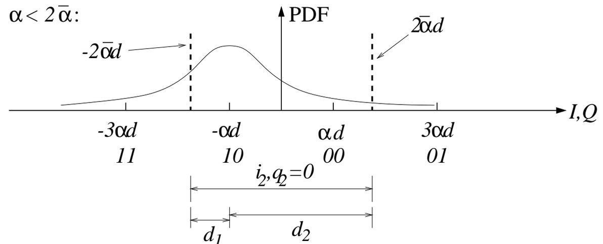
$$P_{2,0,<2}(\alpha) = Q\left(d_1/\sqrt{N_0/2}\right) + Q\left(d_2/\sqrt{N_0/2}\right) = Q\left(\frac{(2\bar{\alpha} - \alpha)d}{\sqrt{N_0/2}}\right) + Q\left(\frac{(2\bar{\alpha} + \alpha)d}{\sqrt{N_0/2}}\right)$$
