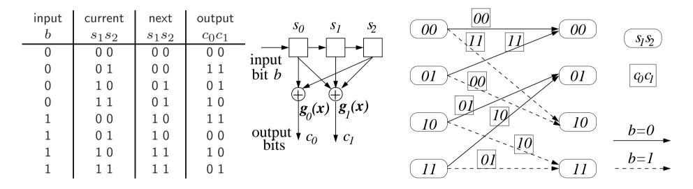
• Only **two legitimate state transitions** for each state, depending on the input bit *b*; similarly, each state has two merging paths; output bits are shown in the box
