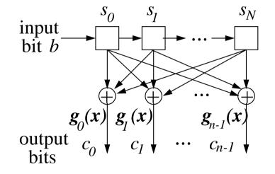
$$g_i(x) = g_{i,0} + g_{i,1}x + \dots + g_{i,N}x^N, \quad 0 \le i \le n-1$$
