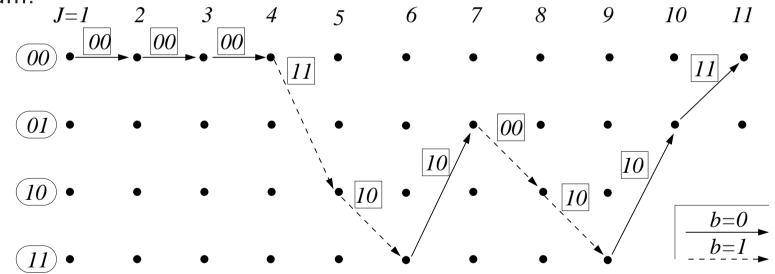
The state is initialised at zero and as the data bit sequence enters, trellis diagram shows the history of state transitions with output bits on it
