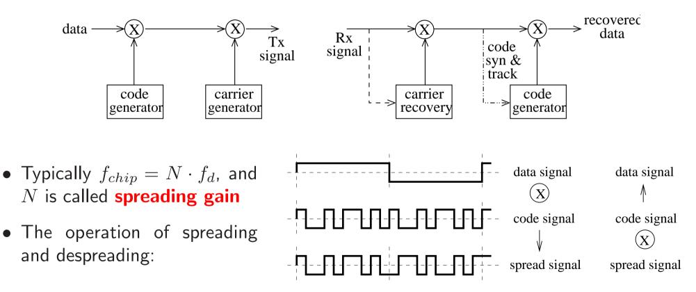
• A key feature of CDMA technology: **spreading sequences** or **codes**
