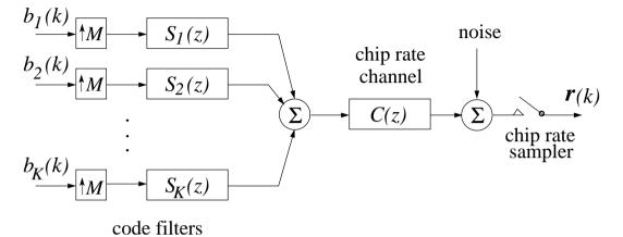
• Assume that there is no multipath distortion, the codes are orthogonal and synchronisation is perfect. Then to detect user i data one only needs to despread  $\mathbf{r}(k)$  with the code  $\mathbf{s}_i$ :
