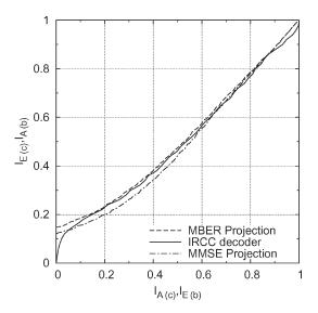
Fig. 4. Projected and optimized EXIT curves of the IRCC for the three-stage iterative beamforming receiver supporting K=6 users with the aid of two antennas at  $E_b/N_0=2~{\rm dB}$ .
