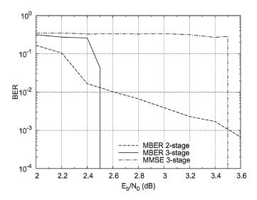
Fig. 6. BER performance of the three- and two-stage iterative beamforming receivers supporting K=6 users with the aid of two antennas.
