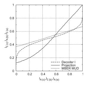
Fig. 3. Two-dimesional projected EXIT charts of the three-stage iterative MBER beamforming receiver supporting K=6 users with the aid of two antennas at  $E_b/N_0=2\,\mathrm{dB}$ .
