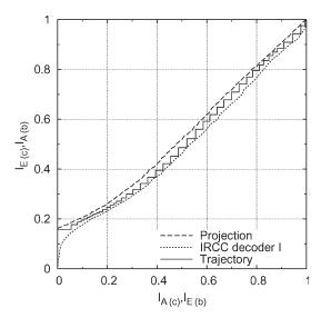
Fig. 7. EXIT charts and recorded iterative trajectory for the three-stage iterative MBER beamforming receiver using IRCCs to support K=6 users with the aid of two antennas at  $E_b/N_0=3.0~{\rm dB}$  over Ricean flat-fading channels.
