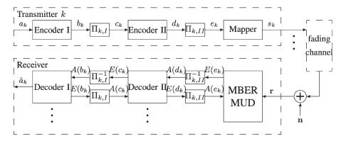
Fig. 1. Three-stage iterative multiuser beamforming system structure.
