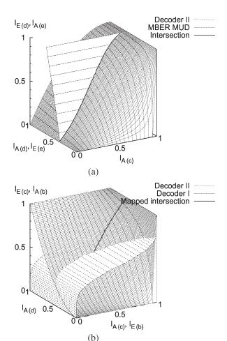
Fig. 2. Three-dimesional EXIT charts of the three-stage iterative MBER beamforming receiver supporting K=6 users with the aid of two antennas at  $E_b/N_0=2$  dB. (a) Decoder II and MBER MUD at  $E_b/N_0=2$  dB. (b) Decoders I and II.
