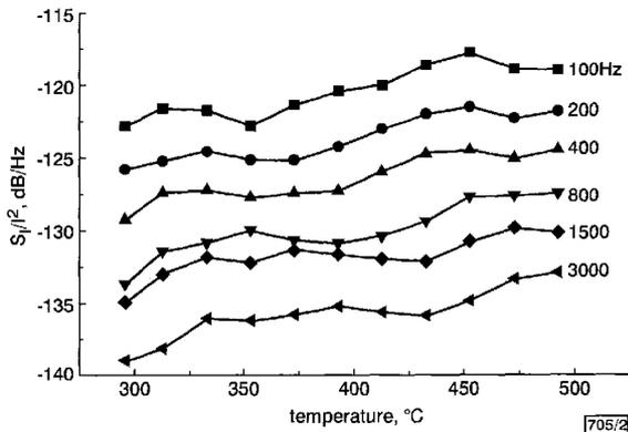
Fig. 2 Temperature dependence of noise  $S_f/f^2$  for MESFET at different frequencies of analysis
