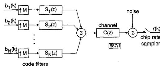
Fig. 1 Discrete-time model of synchronous CDMA downlink
