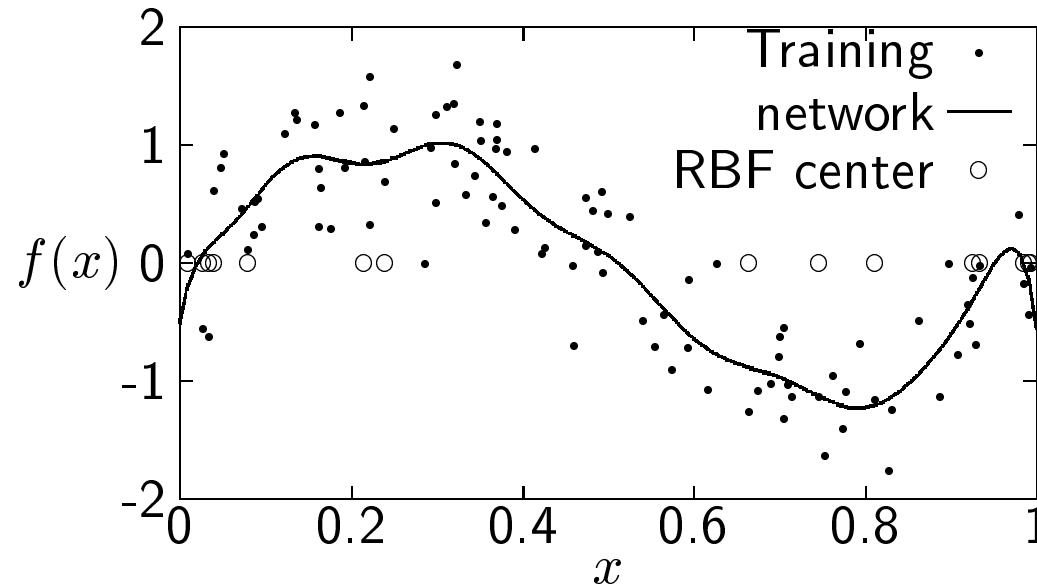
15-term model mapping (curve) produced by the OLS algorithm for the simple scalar function modelling problem. Dots indicate noisy training data  $y$  and circles the RBF centers.
