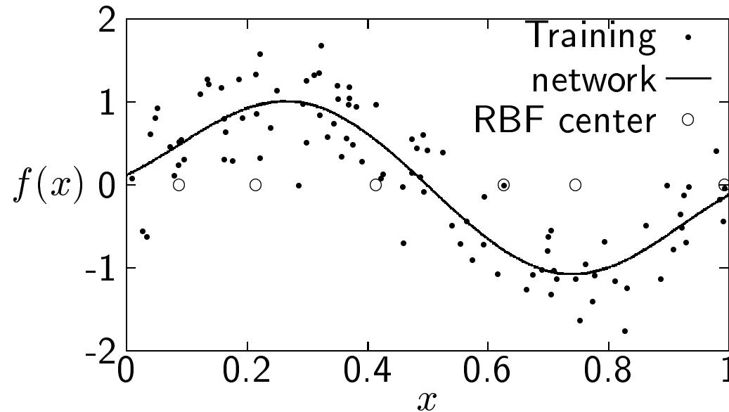
6-term model mapping (curve) produced by the LROLS algorithm for the simple scalar function modelling problem. Dots indicate noisy training data  $y$  and circles the RBF centers.
