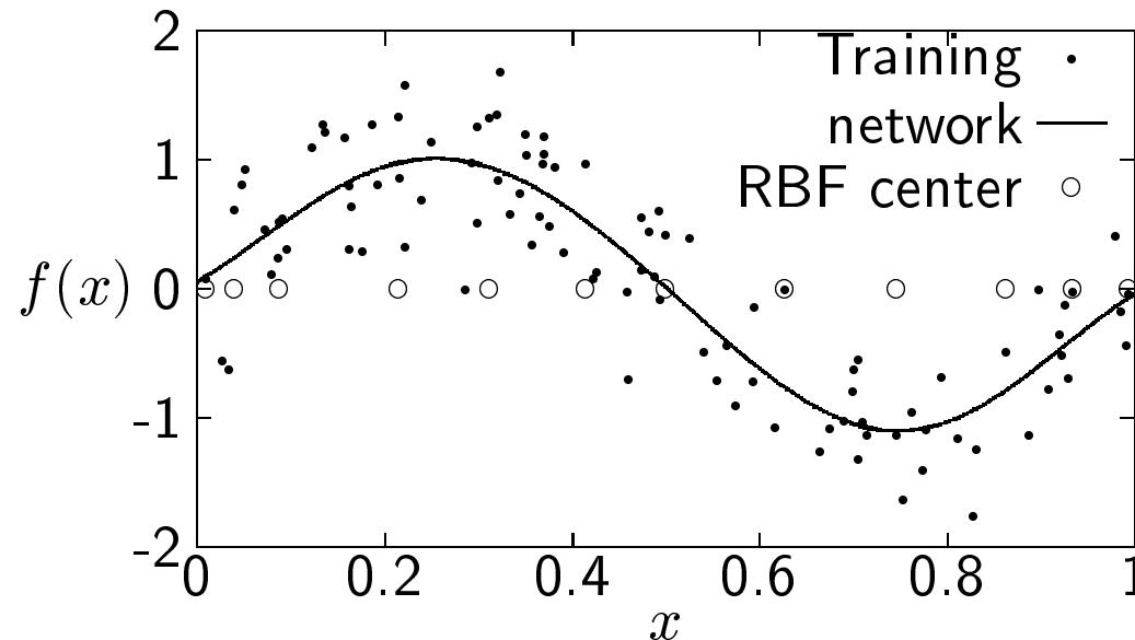
12-term model mapping (curve) produced by the UROLS algorithm for the simple scalar function modelling problem. Dots indicate noisy training data  $y$  and circles the RBF centers.
