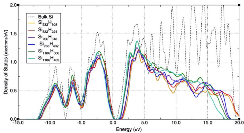
**Figure 6.** Density of states (DOS) of Si<sub>532</sub>H<sub>308</sub>, Si<sub>766</sub>H<sub>402</sub>, Si<sub>1186</sub>H<sub>462</sub>, Si<sub>532</sub>H<sub>224</sub>, Si<sub>766</sub>H<sub>318</sub> and Si<sub>1186</sub>H<sub>366</sub> as calculated with ONETEP [1]. The DOS for bulk silicon (dotted line) has been calculated with CASTEP [34]. In both programs the PBE exchange–correlation functional was used.
