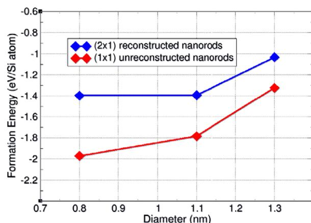
Figure 3. Formation energies of the  $(2 \times 1)$  reconstructed (blue) and  $(1 \times 1)$  unreconstructed (red) nanorods.
