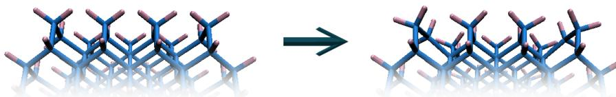
Figure 2. Schematic representation of symmetric hydrogens (before geometry optimization) and 'canted' hydrogens (after geometry optimization) located on a part of the surface of the  $(1 \times 1)$  reconstructed  $\text{Si}_{766}\text{H}_{462}$  nanorod.
