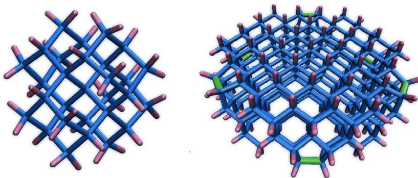
Figure 1. ONETEP optimized structures of  $\text{Si}_{29}\text{H}_{36}$  and  $\text{Si}_{242}\text{H}_{140}$ .
