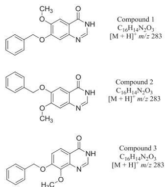
Figure 1. Structures of quinazoline positional isomers.
