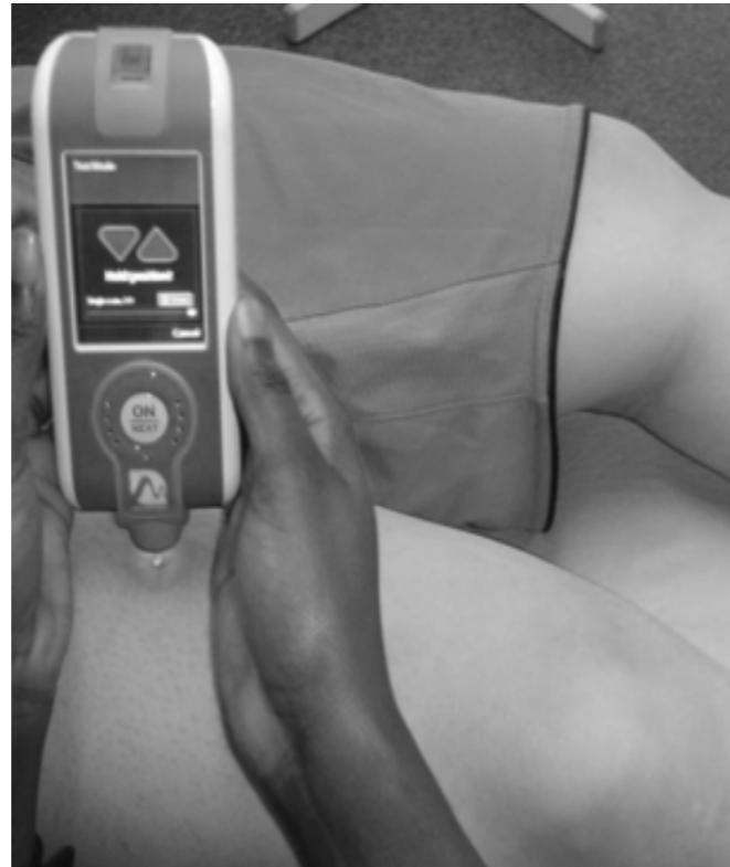
Figure 1 The MyotonPRO device being held perpendicular to the skin over the rectus femoris muscle to obtain measurements of mechanical parameters of non-neural tone, elasticity and stiffness
