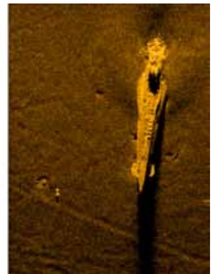
Fig 9 Synthetic aperture sonar principle and image example: German WW2 submarine U-735 submerged in 180m water depth in Oslo Fjord. Image taken at a range of c 200m with a theoretical image resolution of 3 × 3cm. (Image taken by Kongsberg HISAS 1030.)
