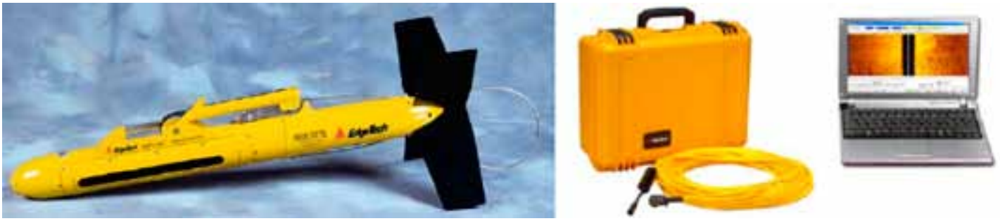
Fig 4 Side scan sonar system (Edgetech 4100 dual frequency).
