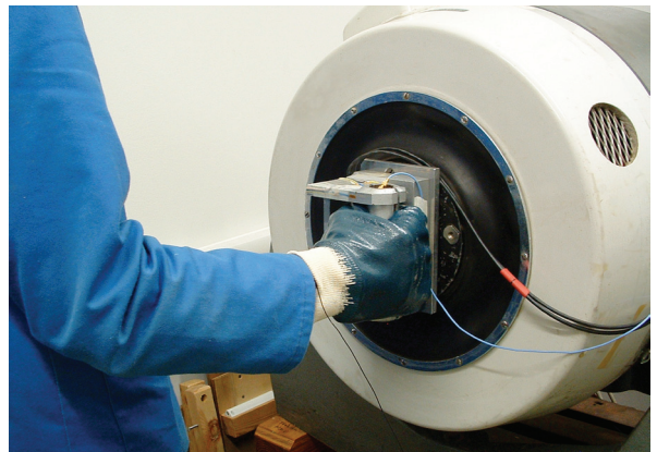
Measurement of transmissibility from a vibrating handle to the palm of a gloved hand
