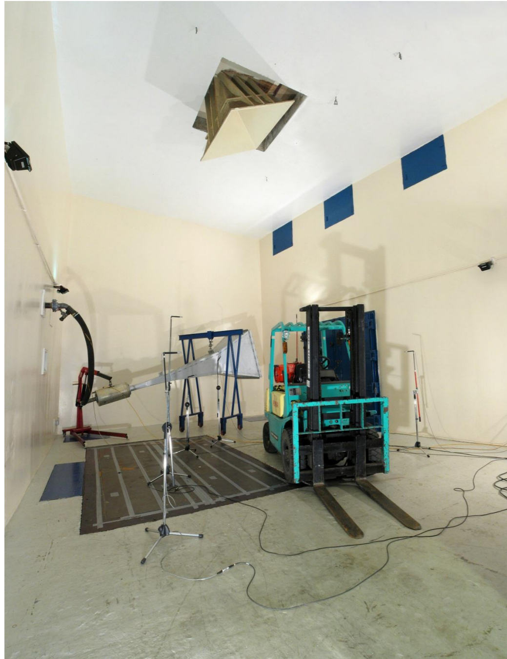
Sound level testing within the Reverberation Chamber
