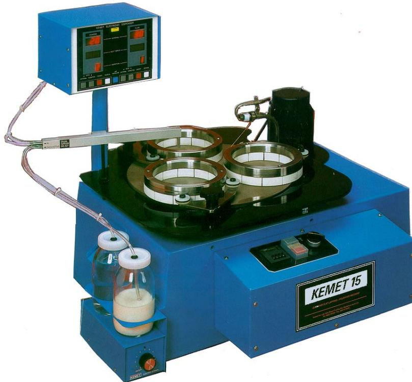
The Kemet 15 is a bench mounted Lapping Machine of rigid metal construction with a Work Table, adjustable for height. It incorporates a digital Process Timer and a fully automatic Liquid Diamond Dispensing System.
