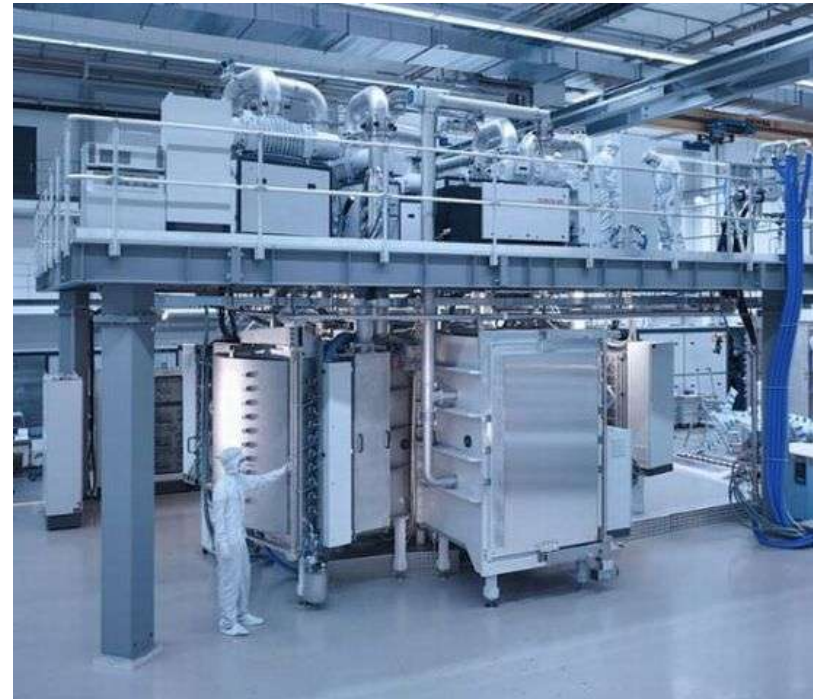
Oerlikon Solar Kai reactor for 1.43m 2 modules
