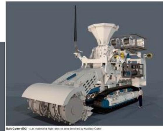
Bulk Cutter (BC) - cuts material at high rates or size selected by Auxiliary Cutter
