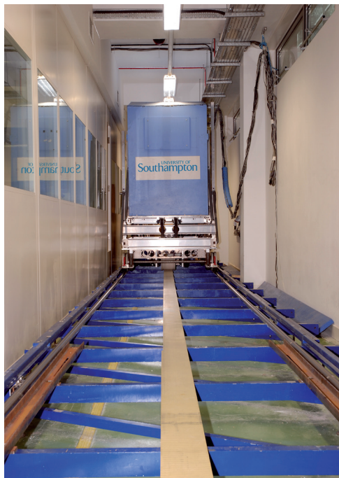
Simulation of lateral and roll, or fore-and-aft and pitch, oscillation in transport environments.
