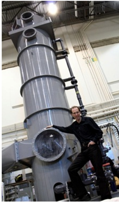
Figure 2.1: Prototype of Air Capturing Tower (source: www.carbonengineering.com )
