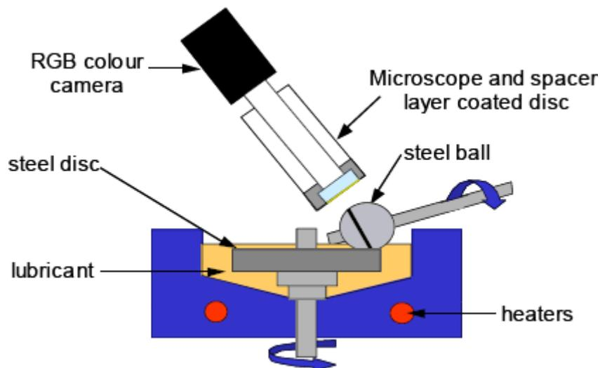
Figure 2: Step 1 – The test ball is run against a steel disc for a pre-defined time
