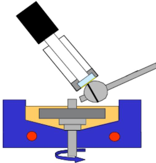
Figure 3: Step 2 – After a pre-defined time, the test Ball is reverse loaded against a coated glass disc and an image is taken The ball is then lowered and the test continues.
