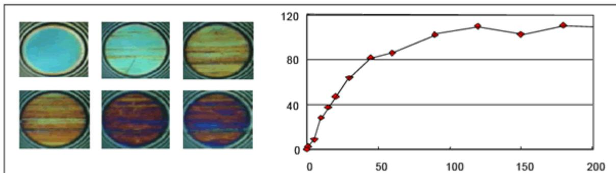
Figure 5: Images (from top left to right) from 0, 5, 20, 30, 90 and 120 minutes running of a fully formulated oil with ZDDP and resulting graph showing ZDDP reaction film thickness (in nm) against time
