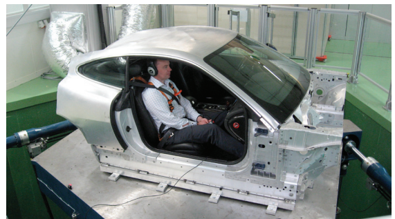
Simulation of 6-axes of motion: vertical, fore-and-aft, lateral, roll, pitch and yaw
