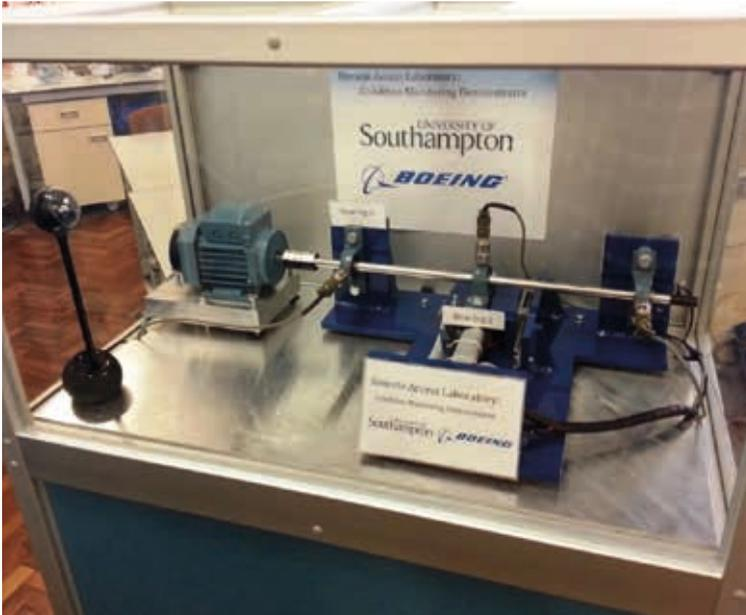
This tool can be used in teaching modules related to a wide range of industries essentially demonstrating sensing and bearing monitoring techniques.
