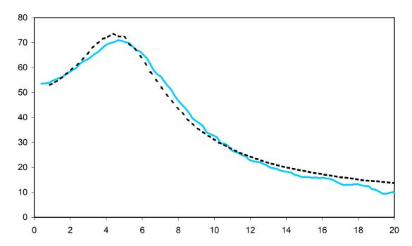
Measured apparent mass of anthropodynamic dummy measured using broadband random vibration at 1.0 ms-2 r.m.s. compared to the Fairley and Griffin model (1989): Measured response, modelled response, modelled response,
