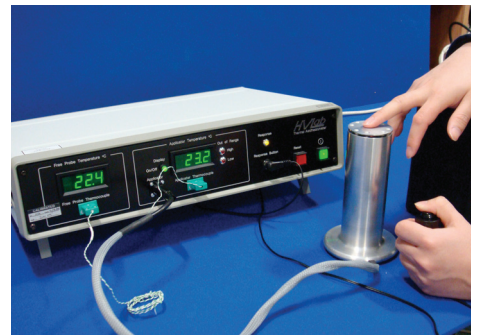
Measurement of thermotactile thresholds at the finger
