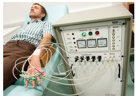
Finger systolic blood pressure measurement
