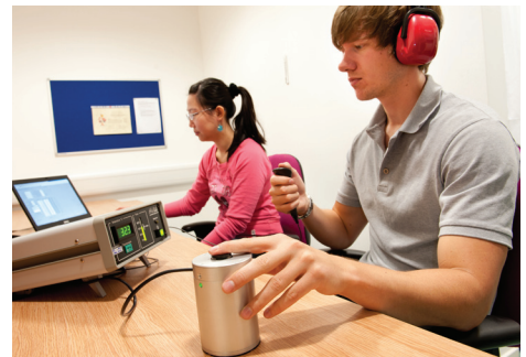
Vibrotactile perception threshold measurement
