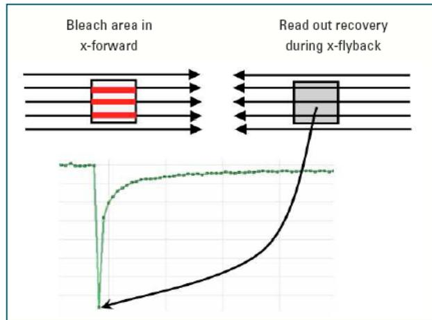
a method to study the rate of diffusion of fluorescent molecules in fluid media (cytoplasm, membranes etc.)
