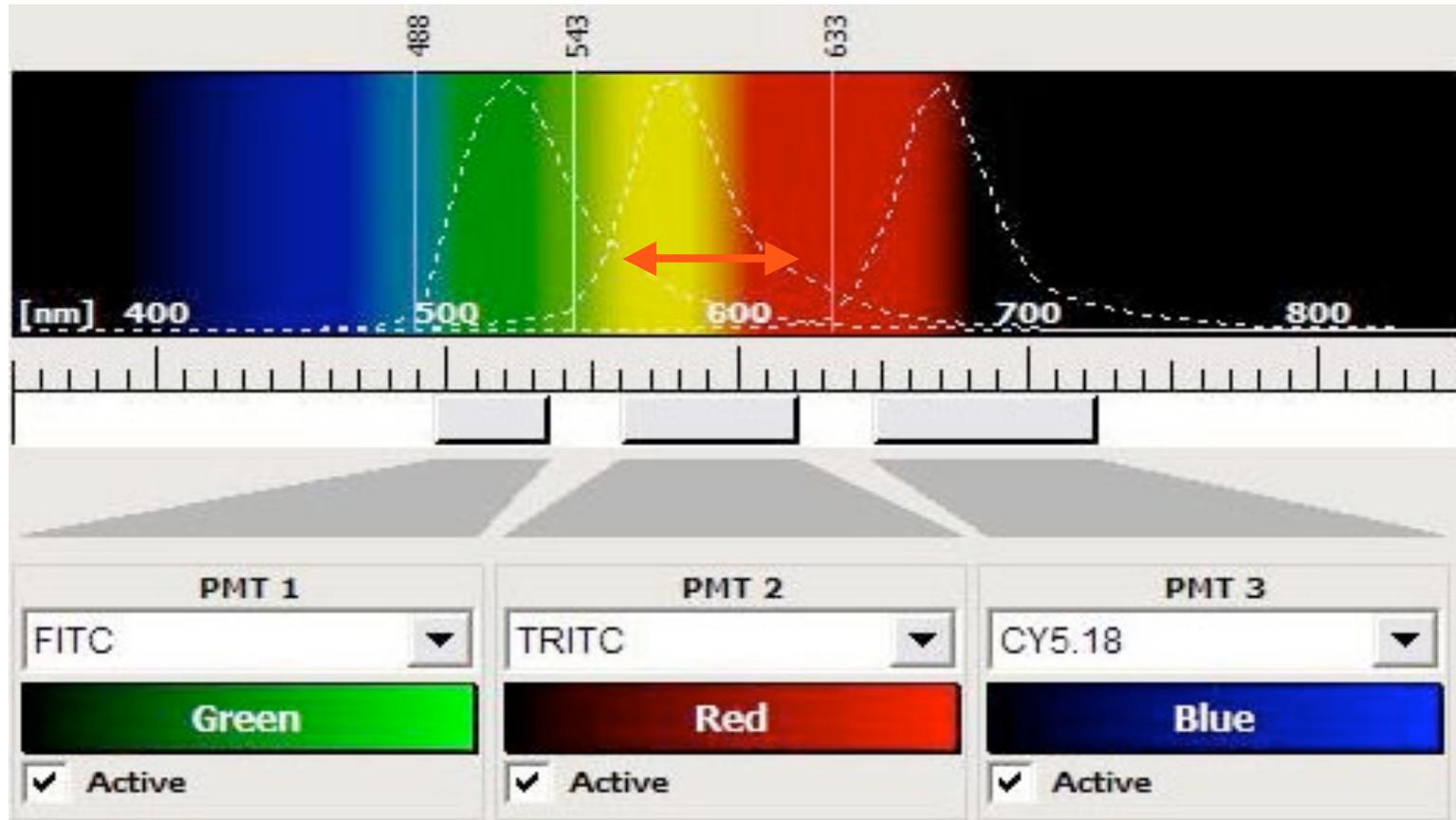
RH tail of FITC fluorescence falls within spectral region being monitored for TRITC fluorescence, ditto (to a lesser extent) for RH tail of TRITC fluorescence in CY5 detection region
