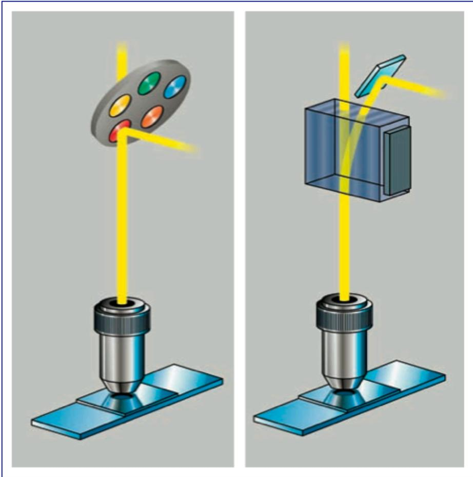
AOBS acts like a dichroic beam splitter to separate shorter wavelength / higher energy reflected excitation from longer wavelength fluorescent emission
