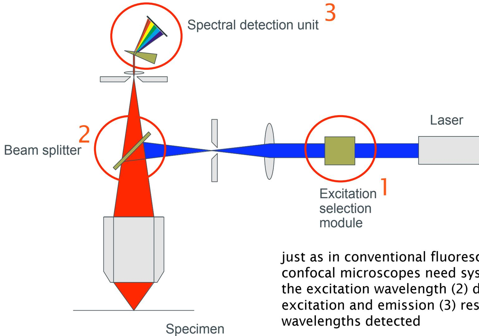
just as in conventional fluorescence microscopy, confocal microscopes need systems to: (1) select the excitation wavelength (2) discriminate between excitation and emission (3) restrict the wavelengths detected
