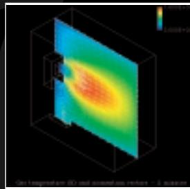
The discrete transfer radiation model solves the radiative transfer equation throughout a domain by a method of ray tracing from surface elements on its boundaries. Solutions
