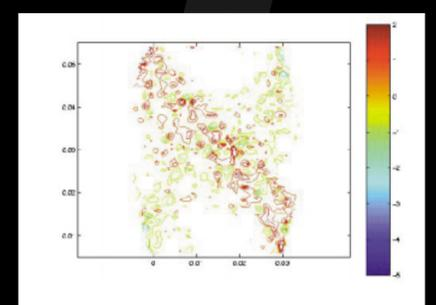
The first three pictures above show the sample after being compressed 2mm, 6mm and 10mm, respectively. The sample can be seen building up barrelling as the test being carried on. The particle rotation pattern is shown in the picture above. It is clear that the deformation is localized and concentrated in two narrow zones.
