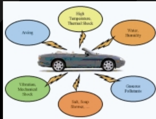
Figure 1: Stresses on Electrical Contacts in an Automotive Environment
