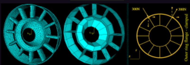
Fig. 1: Fine and coarse meshes, boundary conditions and loads.
