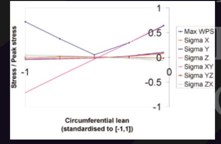
Selecting the 6 stress components at each surface node as an I.R.F. provides a significant reduction in the number of SC03 analyses required to identify the optimum design.
