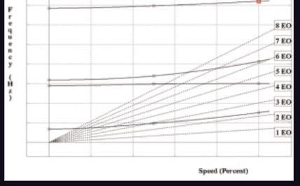
The aerofoil shape was modified by varying the chord at 3 sections and the maximum thickness at 5 sections, using JC14. In this problem I.R.F.'s were introduced to model the frequency for each mode at 3 speeds. The Campbell diagram may then be recreated based on the approximate frequency data to determine the engine order and modal separations.
