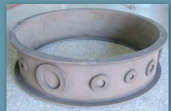
Figure 3: A full sized combustor casing (front case) manufactured by the Powder Hot Isostatic Pressing process
