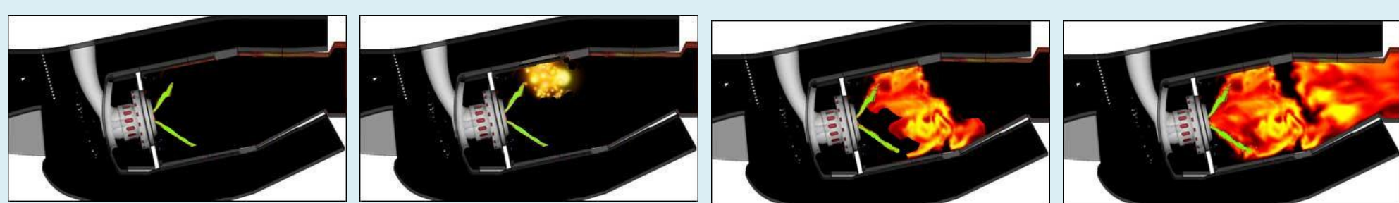
Illustration of a gas turbine combustor ignition sequence, superimposed on a combustor image from Stanford CTR.
