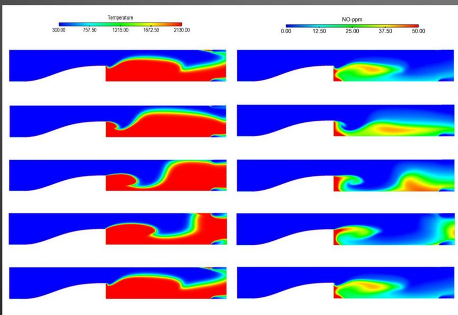
Figure 3. Humming instability cycle (left) and corresponding NOx variation (right) during the cycle (URANS @  $\Delta t = 1e-05s$ )
