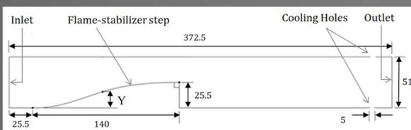
Figure 1. Computational domain of the combustor (All dimensions in mm)
