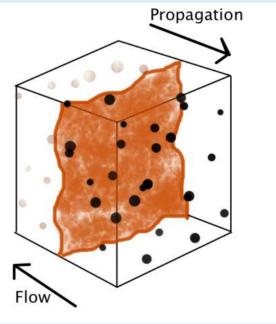
Figure 1: Schematic diagram of DNS configuration, showing a flame sheet propagating in to a turbulent spray.
