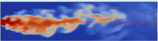
Figure 3: Cross section of the mixture fraction field from a 3-dimensional LES of spray, at two different times.
