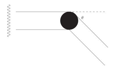
The wave that passes over the nucleus travels a distance  $2R \sin \theta$  further than the wave that passes below the nucleus. If this difference is equal to  $\lambda/2$ ,  $3\lambda/2$  ··· then we get destructive interference. At these angles the differential cross-section vanishes.
