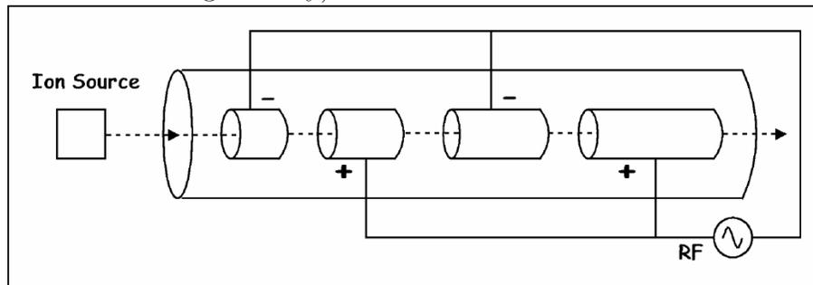
Particles always travel in vacuum. There is no field inside the drift tubes. External field between ends of tubes changes sign so proton always sees  $-ve$  in front and  $+ve$  behind. Proton linacs of 10-70m give energies of 30 to 200 MeV. Usually used as injectors for higher energy machines. Above a few MeV, electrons travel at speed of light. The 'tubes' become uniform in length and microwaves provided by Klystrons provide accelerating potential.
