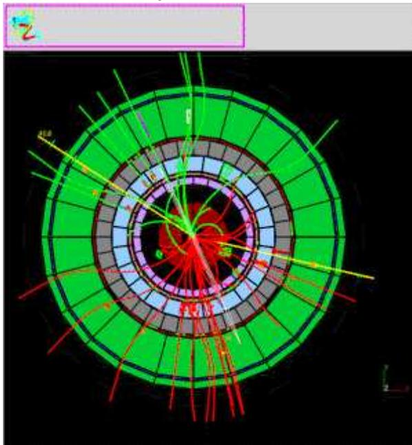
By tracking which of the wires discharge it is possible to reconstruct the paths of the charged particles.
