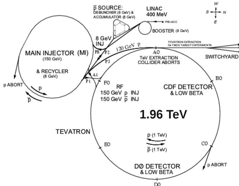
Situated just outside Chicago this is now running the Tevatron in which protons and antiprotons are each accelerated to an energy of 1.96 TeV and then move around a ring of circumference 6 km. This is a synchrotron in which very high magnetic fields are achieved using superconducting (electro-)magnets, which are capable of maintaining very large currents thereby producing large magnetic fields. The luminosity is
