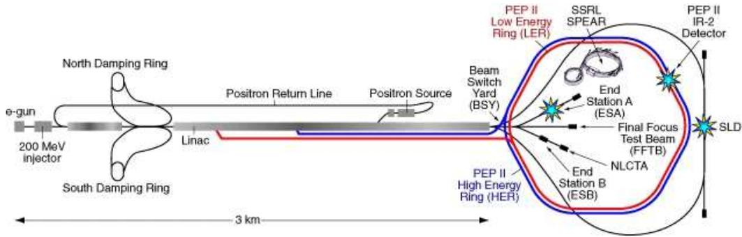
At the end of the tube the electrons and positrons are stored in a storage ring (they go around the storage ring in opposite directions under the influence of the same magnetic field) and there are intersection points where electron-positron scatterings occur.
