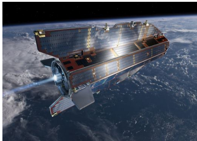
Figure 3. GOCE (Gravity field and steady-state Ocean Circulation Explorer) VLEO Satellite
